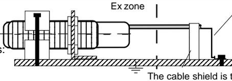
The end of the cable must be connected outside the hazardous location. Check the reliable, noncorrosive holding of the protection earth connection.
